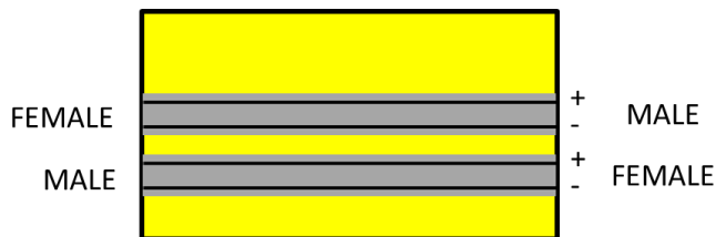
Back of module showing terminal block for hooking up power packs
