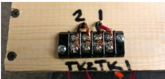
Back of module showing terminal block for hooking up power packs
